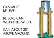
To make measuring Jar, Pour 1" of Water In The Juice Can. Then Pour IT in a Tall Olive Jar and Mark 1". Divide Into Tenths.
